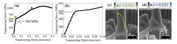
**Figure 8 a** Engineering stress–strain curve for Pillar C from microcompression testing, with a zoomed view provided in (b). The red dashed line represents the 0.2% offset with the yield strength value indicated on the Y axis in each as  $\sigma_{v}$ . **c** and **d** are
