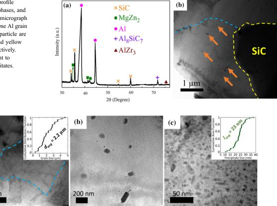
**Figure 4** Bright field TEM micrographs of the Al matrix. **a** One Al grain is outlined in blue dashed lines, and the inset is a cumulative distribution function of the grain size with an average of 2.2  $\mu$ m. **b** Precipitates of various sizes ranging from tens to
