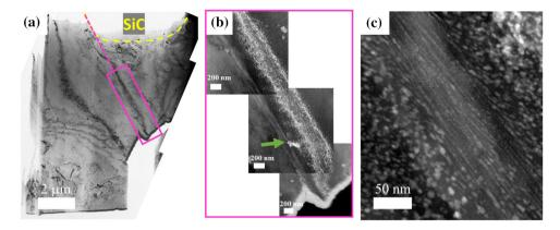
**Figure 10** a Bright field TEM micrograph of the deformed Pillar B. The SiC particle is outlined by a dashed yellow line, which also represents the matrix–particle interface. The area outlined by a purple box shows a dominant shear band, which is shown in more detail in (b). The dotted purple line follows the trace of the dominant shear band, which aligns well with the matrix–particle
