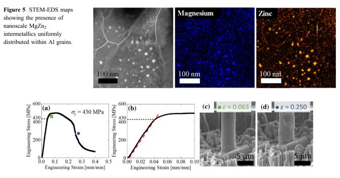
Figure 6 a Engineering stress-strain curve for Pillar A from microcompression testing, with a zoomed view provided in (b). The red dashed line represents the 0.2% offset with the yield
