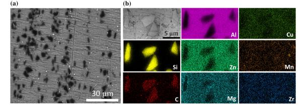
Figure 2 a Backscattered electron SEM micrograph of the composite surface, which shows SiC particles (dark regions) and intermetallics (light regions) distributed in the Al matrix. **b** A
