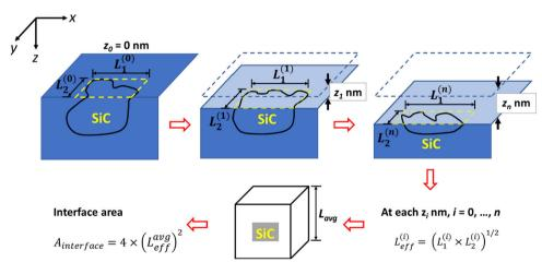
**Figure 12** Schematic illustration of measuring particle sizes via post-test milling at different depths. A rectangular is used to enclose the shape of the particle on the top surface (x–y plane) at each depth  $z_i$ , and the side lengths are  $L_1^{(i)}$  and  $L_2^{(i)}$ . Then, an effective length at each  $z_i$ ,  $L_{eff}^{(i)}$ , is obtained by taking the square root of the product of  $L_1^{(i)}$  and  $L_2^{(i)}$ . The shape of the particle is
