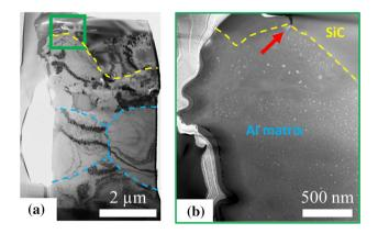
Figure 9 a Bright field TEM micrograph of the deformed Pillar A. SiC particle and Al grain boundaries are outlined by yellow and blue dashed lines, respectively. A region containing a crack that has arrested at the matrix—particle interface is enclosed by a green square and magnified view is shown in **b**. The exact location of crack arrest is denoted by a red arrow at the matrix—particle interface.
