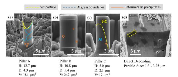
**Figure 1 a**–**c** SEM micrographs of three pillars with different microstructures and **d** two perpendicular surfaces milled to reveal a SiC particle. H, D, and V correspond to height, diameter, and
