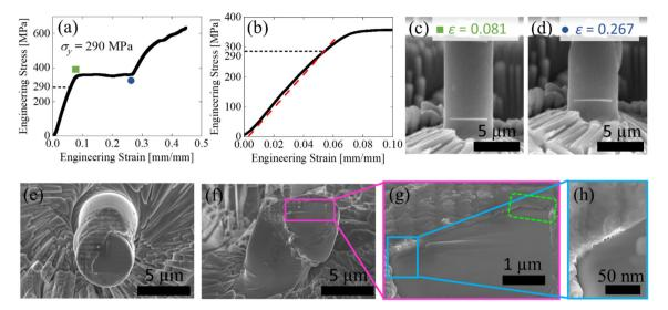
**Figure 7 a** Engineering stress–strain curve for Pillar B from microcompression testing, with a zoomed view provided in (b). The red dashed line represents the 0.2% offset with the yield strength value indicated on the Y axis in each as  $\sigma_y$ . **c** and **d** are SEM snapshots corresponding to engineering strains of 0.081 and 0.267, respectively. **e** Top view of the deformed pillar, which clearly shows matrix–particle interface debonding. **f** Side view of
