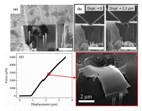
Figure 11 a Two perpendicular surfaces containing one SiC particle are created using FIB milling. b A load is applied on the particle using a slightly rounded tip until the particle separates from the matrix. The corresponding displacements are shown for the two images. c Representative force–displacement data from a direct debonding test. The obvious drop in the force does not
